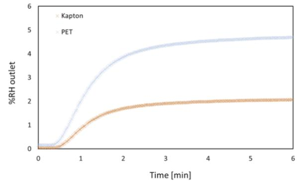
Figure 2. The comparison of water permeation on Kapton and PET
