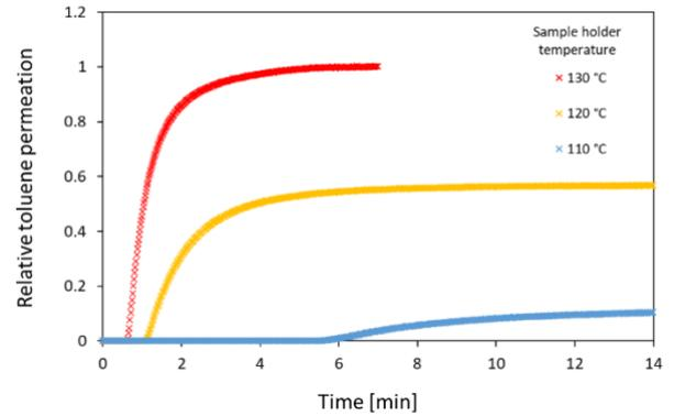
Figure 4. Analysis of toluene permeation in PET at 110 °C, 120 °C and 130 °C, relative to equilibrium permeation at 130 °C.
