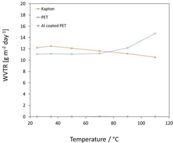
Figure 3. The glass transition effects on Kapton, PET, and multi-layered aluminium PET using water
