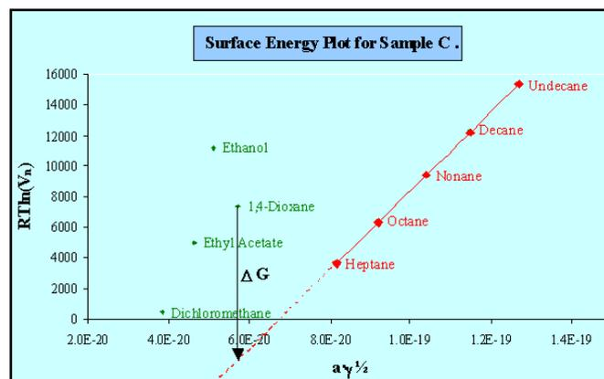
Figure 1. Dispersive surface energy plot (in red) and specific free energy of desorption for several polar probe molecules (in green) eluted through a column of batch C. 0% RH, 30 °C, 0.03P/P<sub>0</sub>.
