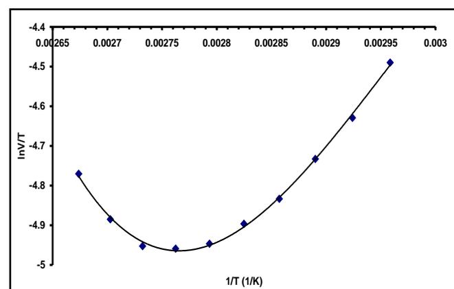
Figure 7. Glass transition results on a  $\alpha$ -D-Maltose monohydrate sample.
