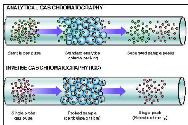
Figure 2. Schematic of *iGC SEA* principle.
