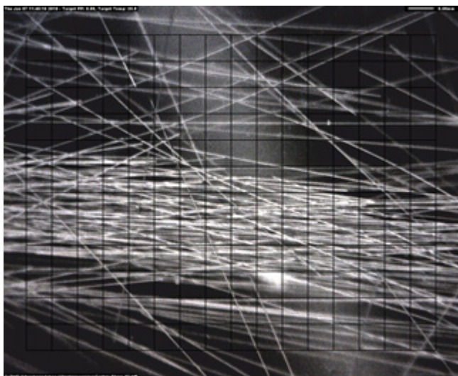
Figure 6 – Carbon fibers at 200X, with grid overlay.
