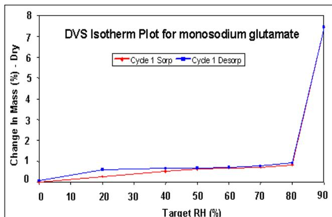
Figure 2. Water sorption isotherms for monosodium glutamate at 25 °C
