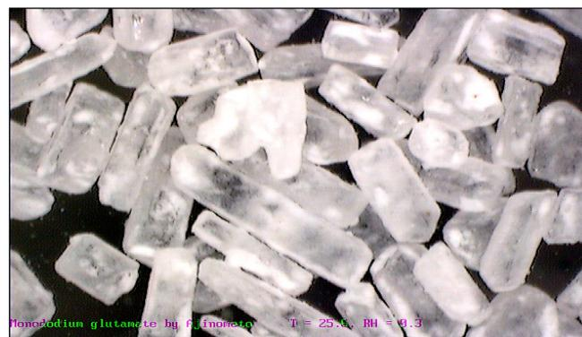
Figure 3. Video microscopy output on monosodium glutamate at 0%RH and 25 °C.
