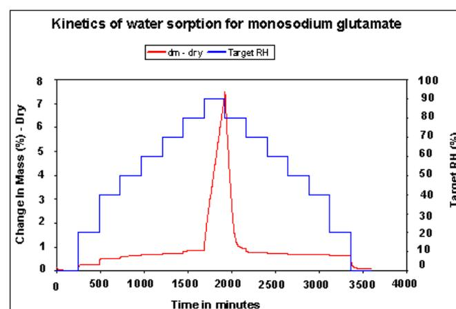
Figure 1. Kinetics of water vapour sorption for monosodium glutamate at 25°C
