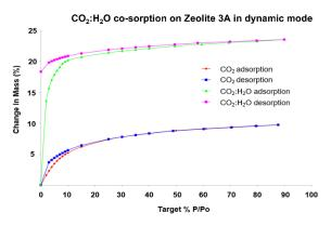
Figure 6: CO<sub>2</sub> sorption and Co-adsorption of CO<sub>2</sub> / water (10:1) sorption on Zeolite 3A
