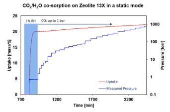
Figure 5: CO<sub>2</sub> adsorption on humid Zeolite 13X
