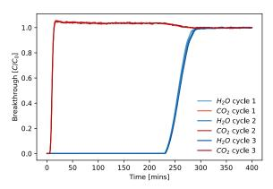
Figure 11: Three repeated breakthrough curves of  $CO_2$  (3.5%) and  $H_2O$  (20%  $P/P_0$ ) on a sample of Zeolite 13X
