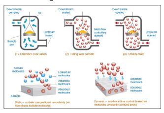
Figure 1. Principle of dynamic vacuum method.
