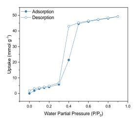
Figure 7. Water adsorption and desorption isotherms of the functionalised material MIL-101(Cr)-4F (1%)
