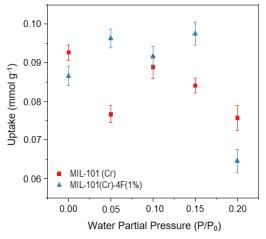
Figure 10. Carbon Dioxide (CO<sub>2</sub>) adsorption capacities of MIL-101(Cr) and MIL-101(Cr)-4F(1%), CO<sub>2</sub>  $P/P_0 = 0.05$  at different water partial pressures (0, 0.05, 0.1, 0.15 and 0.2  $P/P_0$ ) at 298 K and 1 bar.
