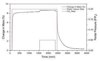
Figure 9. Adsorption and desorption mass change of MIL-101(Cr) exposed to a step change of water partial pressure of 0.2 P/P<sub>0</sub>, followed by a CO<sub>2</sub> partial pressure step change of 0.05 bar at 298 K and 1 bar total pressure.
