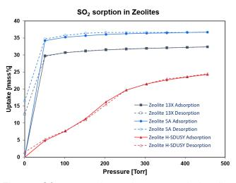
Figure 4. SO<sub>2</sub> gas sorption on three prototypical zeolites
