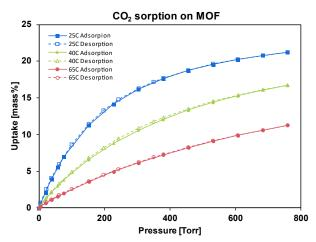
Figure 2: CO<sub>2</sub> gas sorption on MOFs
