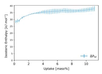
Figure 3: Enthalpy of adsorption of CO<sub>2</sub>
