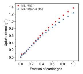
Figure 8. Carbon dioxide (CO<sub>2</sub>) adsorption isotherms at 298 K and 1 bar of MIL-101(Cr) and MIL-101(Cr)-4F(1%).
