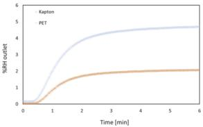
Figure 2. The comparison of water permeation on Kapton and PET
