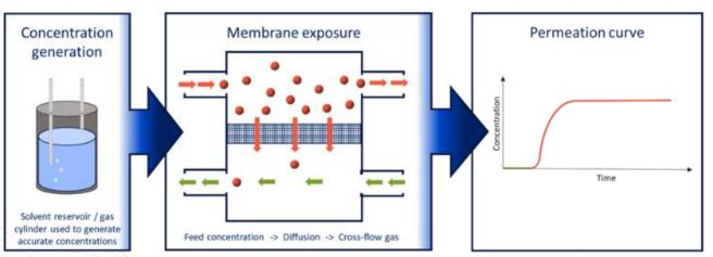
Figure 1. Schematic of the basic principles of the MPA
