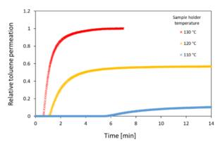
Figure 4. Analysis of toluene permeation in PET at 110 °C, 120 °C and 130 °C, relative to equilibrium permeation at 130 °C.
